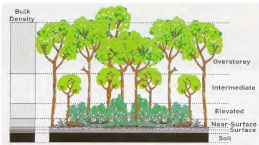
Figure 1: The five fuel layers in a forest environment that could be associated with fire behaviour (Gould et al. 2007)
